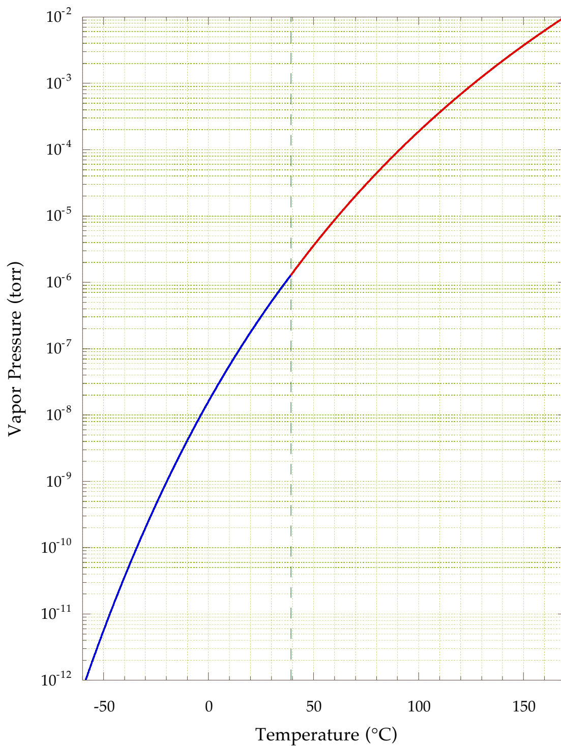
Figure 1: Vapor pressure of ^{87}\text{Rb} from the model of Eqs. (1). The vertical line indicates the melting point.
